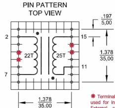
\* Terminals 3, 4, 13 & 14 are used for internal connections. External circuit connections must provide appropriate isolation for these terminals.
