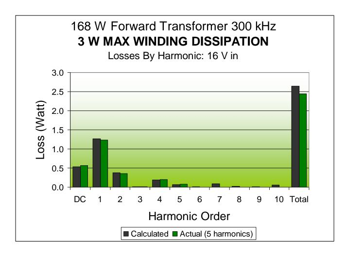
Hyper-X Magnetic Technology was used to determine winding losses layer by layer and to determine the configuration of a redesign using distributed optimization. This optimization process considered both DC and AC current components using harmonic decomposition of the application wave shapes. Harmonic test methods carefully correlated actual loss within 5% of calculations.
