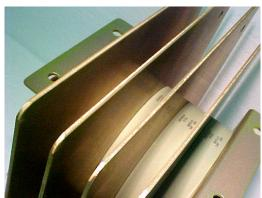
The "K" series integrates metal fins into the disk resistor stack to improve forced or freeair convection cooling, obtaining a higher average power rating. This technique also reduces cool-down time in crowbar or dump applications when repetitive operation is a requirement.
